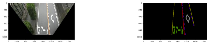
Figure 4. Example of the obtained BEV images (left: original image; right: segmentation result).
