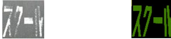
Figure 5. Example of the obtained road marking images (left: original image; right: segmentation result).
